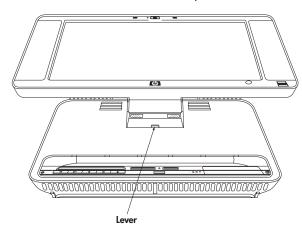
4 While holding down the lever, pull the vertical cover up and remove from the chassis.
