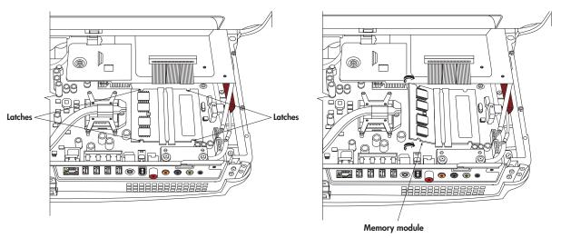
**6** Lift the memory module from the memory socket. Note the location of the key slot on the connector edge.
