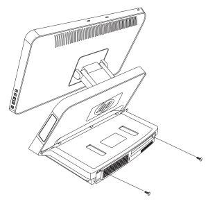
3 Pull the rear cover back about 1/2 in (1.27 cm) (A). If necessary, gently push down on the cover while pulling back.
