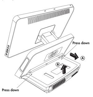
4 Lift the rear cover and remove from the chassis (B).
