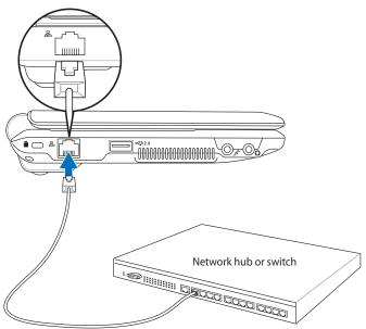
Network cable with RJ-45 connectors
