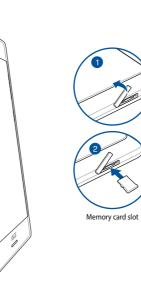
The memory card slot supports microSD, microSDHC, and microSDXC card formats.
