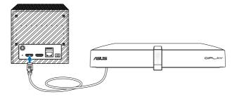
Connect the bundled IR Blaster cable to the IR Blaster port at the back of your ASUS QUBE.
