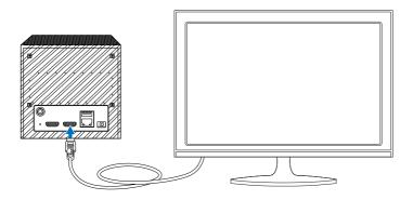
Use an HDMI cable to directly connect your external display such as HDTV to your ASUS QUBE's HDMI-Out port.
