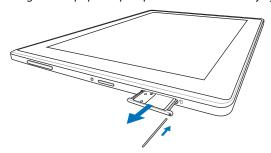
2. Remove the tray from the slot. Orient and place the SIM card on the tray.
