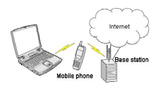
Configuring a mobile telephone for use as a modem Connecting to the Internet
