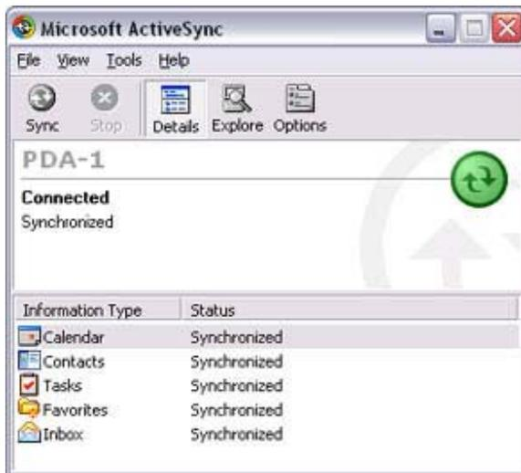
While the ActiveSync connection is active, synchronisation will be performed whenever information is changed on either the PC or the PDA.
