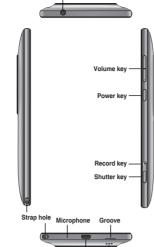
NOTE: Pry open the rear cover from the groove.
