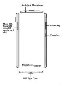
NOTE: The USB Type-C port supports USB2.0 transfer rate.
