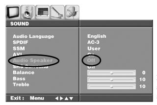
Make sure that the TV speakers are set to OFF when using an external sound device.
