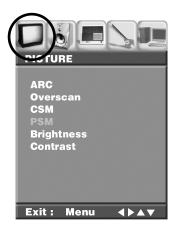
Press the <OK> button or the < > button on the remote control. The menu will be selected, and the submenus can be navigated. Select the 'CSM (Color Standard Mode)' submenu and press the < > button on the remote control to select the option item (select option items like 'Normal, Cool, User, Warm1~2' and so on in the 'CSM' submenu).
