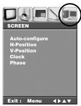
Press the < > button on the remote control to navigate to the 'Auto Configure' submenu, and press the < > button on the remote control. The 'Auto in Progress' screen will be displayed, and the screen will be adjusted automatically.
