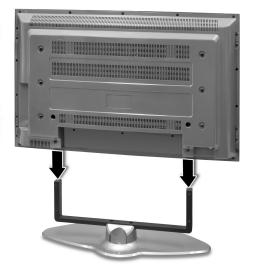
A Secure the LCD TV with screws.
