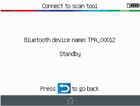
I - Put the TPA 300 into “Connect to scan tool” mode.
