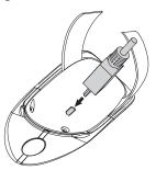
During the charging process, the MF button lights red. After the battery is fully charged, the MF button lights blue. The charging process of the battery lasts approx. 3 hours. Disconnect the BT Drive Free 411 from the charger after it has been charged.
