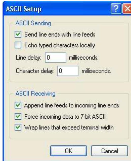
2. You can input word “AT” then press “Enter” key, it should be response word “OK” means work property. **All commands are executed by pressing “Enter” key.**
