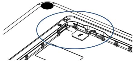
When putting the battery back in place, please make sure both hooks have clicked and are safely secured.
