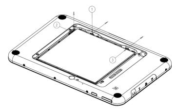
Enter the SIM card into the slot in the bottom right corner. Please make sure you have the SIM card in the correct direction (chip facing down).
