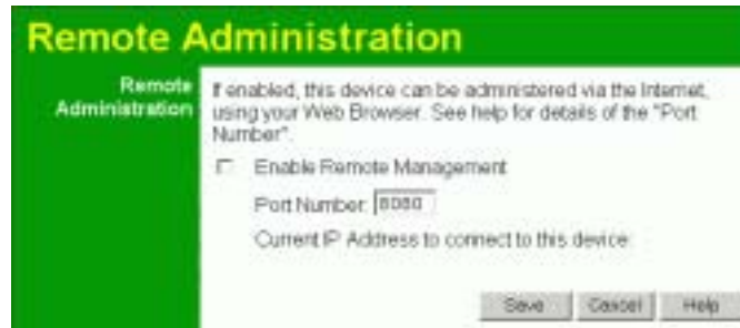
Figure 47: Remote Administration Screen
