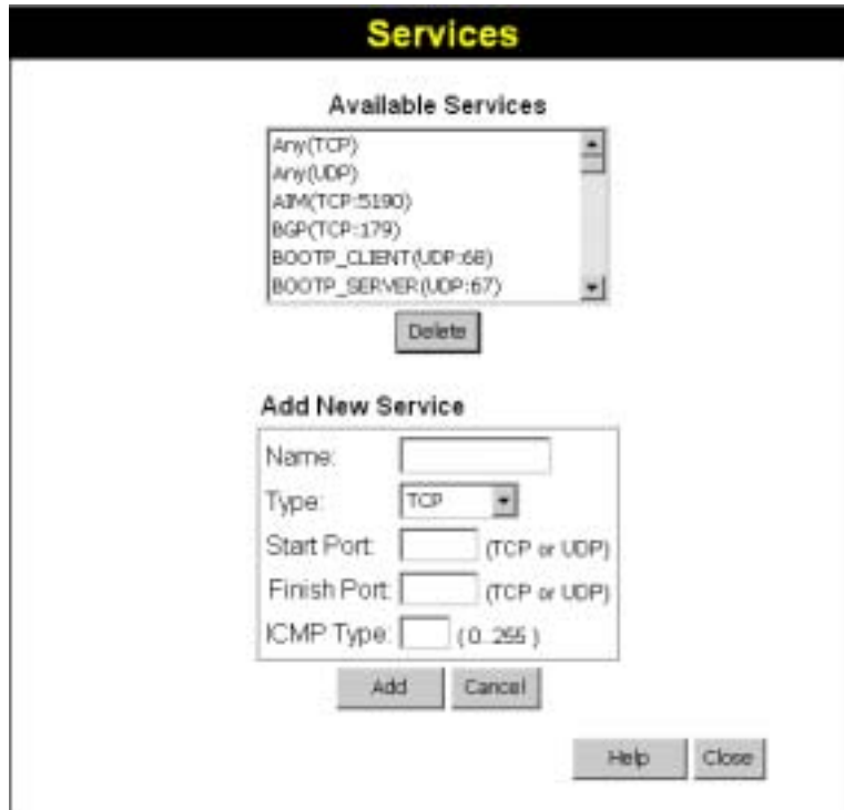
Figure 33: Access Control - Services
