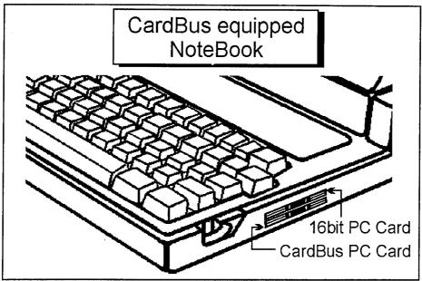
Due to variant design of notebook computers, some models implement a setting in the Computer 's BIOS to switch between Cardbus and 16-bit PC Card modes. You could consult the User's Guide of your notebook and properly set on the CardBus or Auto\_Detect mode.
