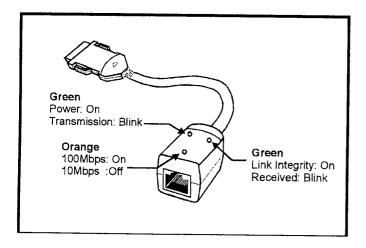
The Fast Ethernet PC Card provides three LEDs for easy diagnosis and installation.
