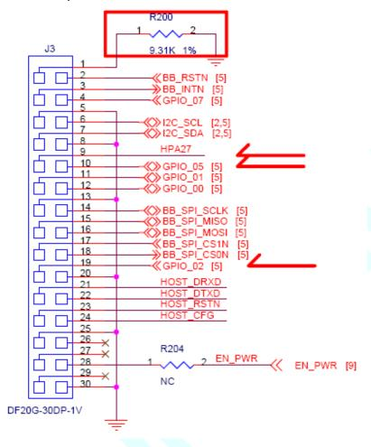
This connector use for manufcture purpose and engineering debug. Connector P/N: DF20G-30DP-1V of Hirose, PVT and MP model will change to P/N MDS24011P15C of STM
