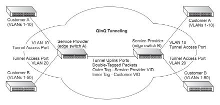
Layer 2 Flow for Packets Coming into a Tunnel Access Port
