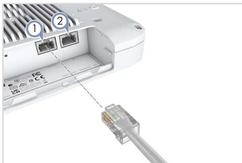
1. Connect Category 5e or better cable to the Uplink (PoE) 1000BASE-T RJ-45 port. When connected to a PoE source, the Uplink (PoE) port connection provides power to the unit.
