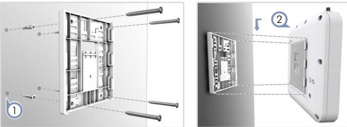
1. At the installation location on the wall, use the mounting bracket to mark four holes for the wall plugs and screws (included in the screw kit).
