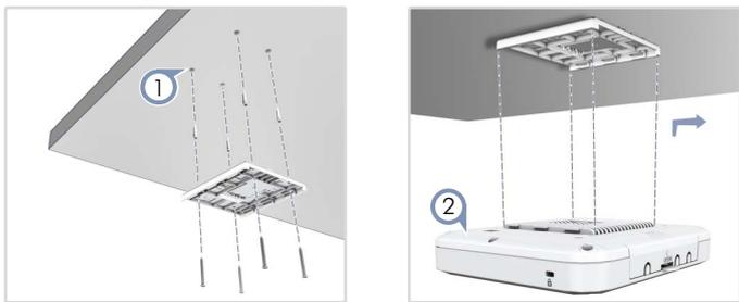
1. At the installation location on the ceiling, use the mounting bracket to mark four holes for the plugs and screws (included in the screw kit). Drill four holes for the plugs, and then insert the plugs and tap them flush with the ceiling surface.
