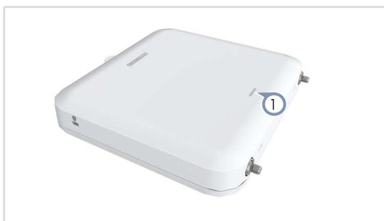
1. When operating normally, the System LED should be on green. Blinking indicates the device is booting up.
