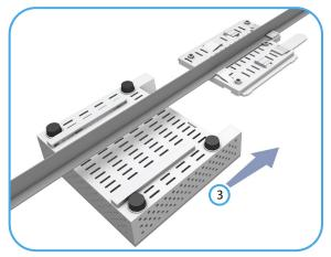
3 Slide the rails on the back of the AP along the sides of the ceiling mounting plate until it snaps into its secured position.
