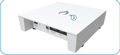
The system/wireless LED should be on red when the AP is powered on, or on/blinking green (2.4 GHz) or blue (5 GHz).
