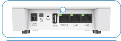
The WAN/PoE port link/activity LED should be on/blinking green. When connected, the LAN1 and LAN2 port link/activity LEDs should also be on/blinking green.
