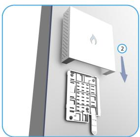
With its ports facing down, place the AP against the wall above the mounting plate.
