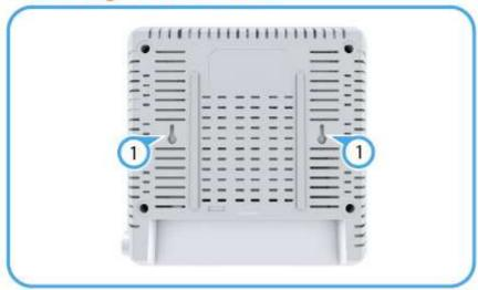
1 At the installation location on the wall, mark two holes 116 mm (4.57 in.) apart for the wall plugs and screws.
