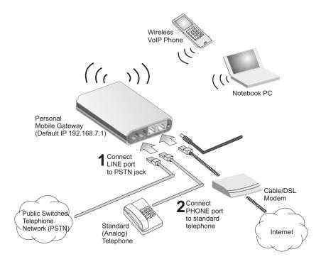
To connect the Personal Mobile Gateway to use its telephony functions, first connect and configure the Personal Mobile Gateway in the operating mode you want to use (see the appropriate section in this chapter.), then follow these steps:
