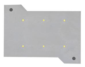
**NOTE**: Care must be taken when using the inside holes. If using the lower left hole as shown above, be sure to use a screw that will not rise above the extruded countersink as this may short the input connector.
