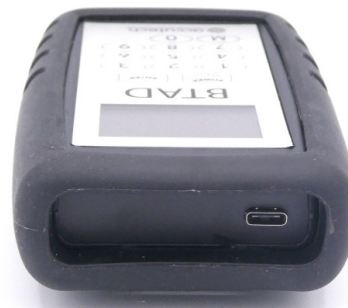
Charging Port on BTAD
