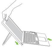
The adjustable kickstand allows the computer to also function as a display that you can control using touch input.
