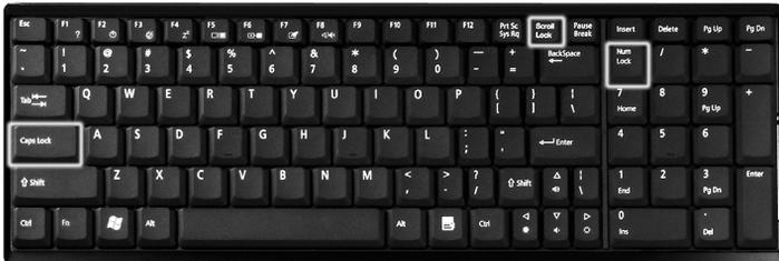
The computer features three lock keys, each with its own status indicator light.
