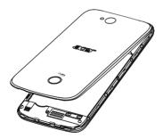
3. Insert the SIM or microSD card as shown.
