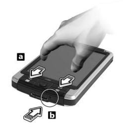
2. While holding the Today and Messaging buttons (**a**), Using the tip of your stylus, lightly press the reset button inside the hole (**b**) on the base of your handheld.
