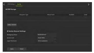
When you connect a USB storage device to the USB port that is specified for NAS functions (USB port 4, by default), users connecting to the LAN network of the Dock will be able to access the files/folders of the USB storage by entering "\\192.168.1.1" or "\\((entryname)") in the URL field. This page displays the status of the connected device that is specified as a NAS.
