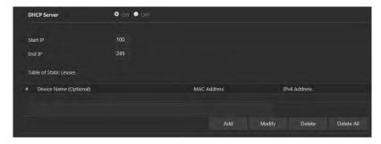
DHCP assigns LAN IP addresses for connected Wi-Fi devices. You can specify an IP address range for the Gateway to assign from.
