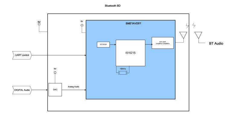
Digital Audio Port: Support I2S format digital audio and DAC will transfer digital audio to analog audio UART Control Port: Support UART command to control Bluetooth board Power Supply: Support 5V power supply
