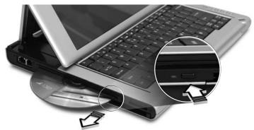
When the power is off, you can eject an optical disk by inserting a pin or paper clip into the emergency eject hole.
