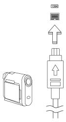
The computer's IEEE 1394 port allows you to connect to an IEEE 1394 supported devices like a DVD/CD-RW combo or DVD-Dual drive.
