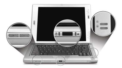
The battery, media and wireless communication status indicators are visible even when the LCD display is closed.
