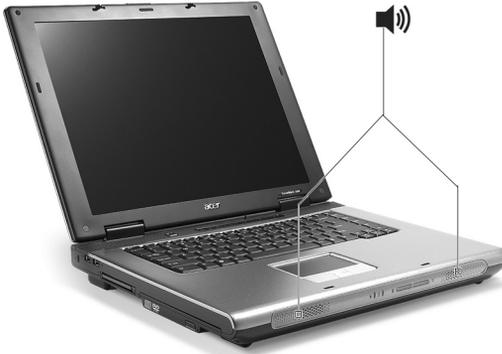
Volume is adjusted using software, such as Volume Control in Windows, Volume **Fn** keys, or any other application that provides a volume adjustment control.
