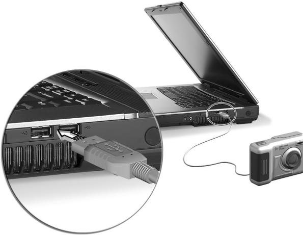
USB is plug and play, which means that you can connect and start using a USB device without having to restart your computer. You can also disconnect the device at any time.
