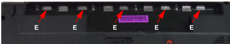
Figure 3-4. Lower Cover Slots
