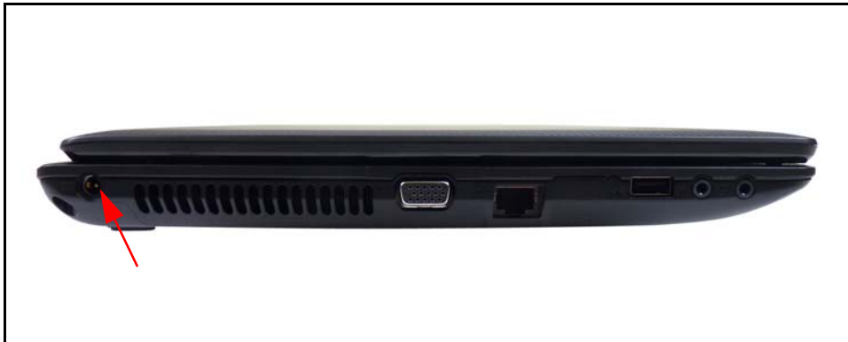
Figure 3-2. AC Adapter Outlet
