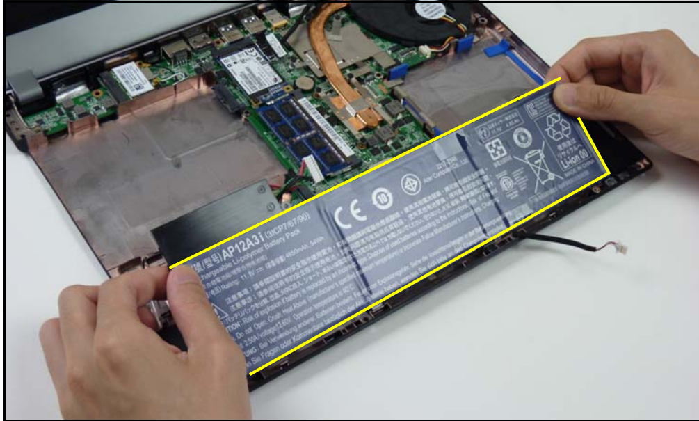
Figure 3-1. Battery Pack Installation
