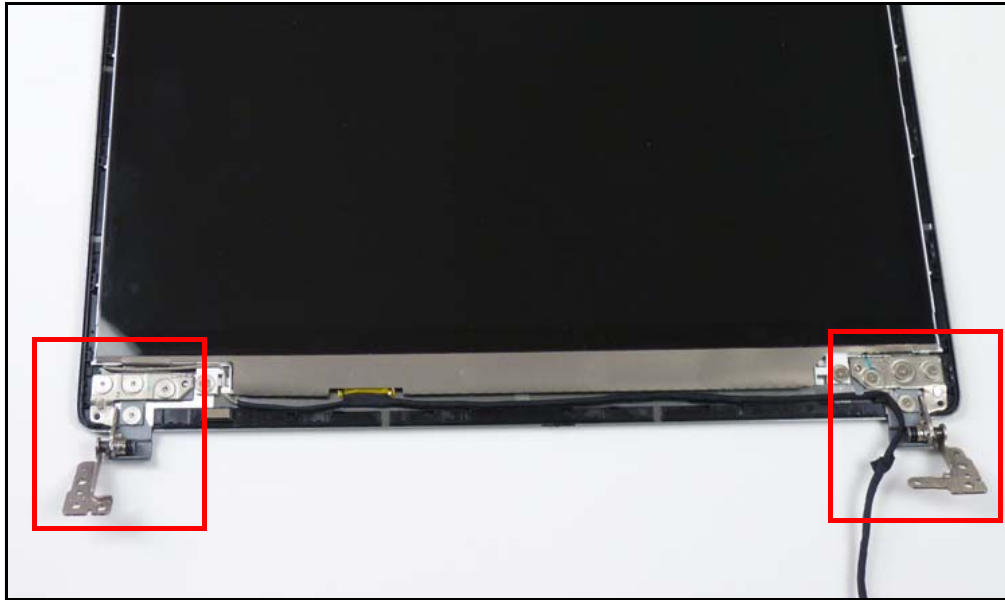
Figure 3-1. LVDS Cable Removal
