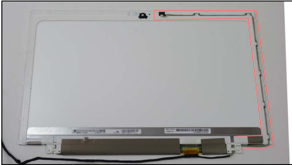
Figure 3-1. LVDS Cable Removal
