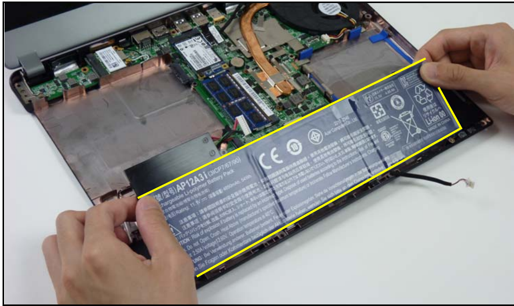
Figure 3-3. Battery Battery Removal
