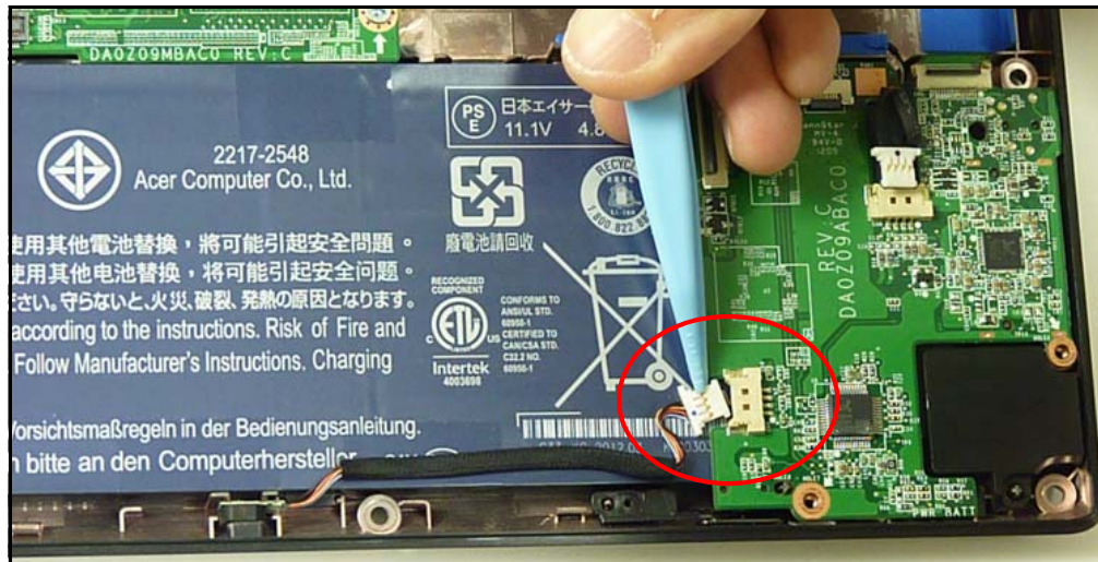
Figure 3-1. MIC Cabling Removal
