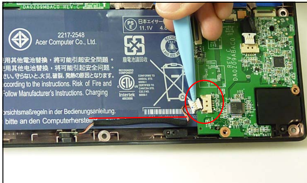
Figure 3-2. MIC Cable Connection
