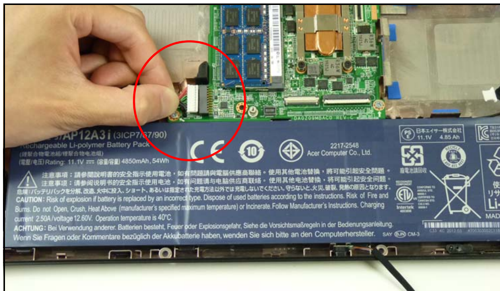
Figure 3-2. Power Cable Removal
