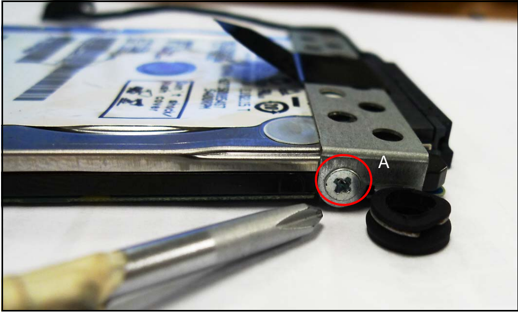
Figure 3-1. HDD Bracket Installation
