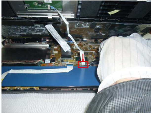
Figure 3-116. Touch Pad Cable
