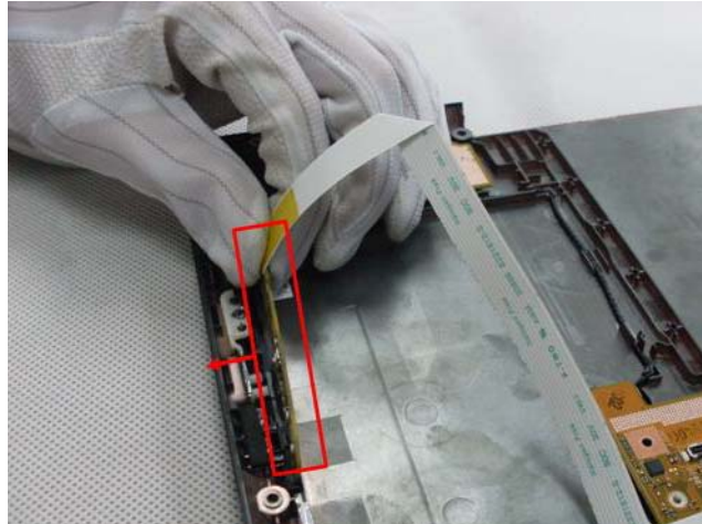
Figure 3-38. Power Switch Board
