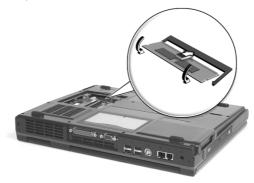
4 Replace the memory compartment door, and fasten the screw. The computer automatically detects the new module and reconfigures the memory.
