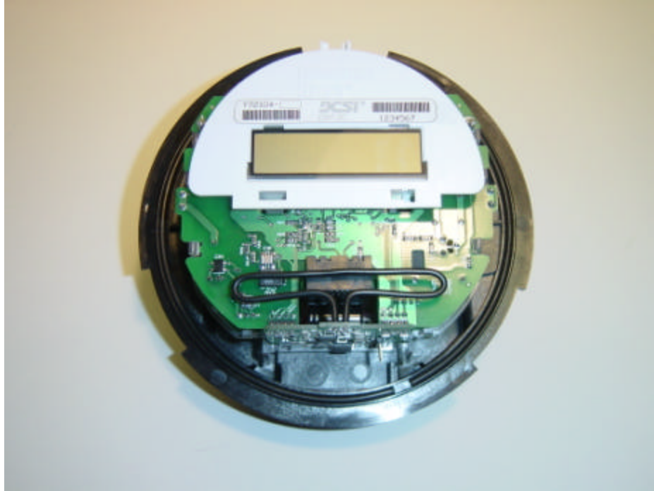
Figure 7 - EMT-3C-MP board hosting the Centron's LCD/Metering Components and the EMTR RF Board
