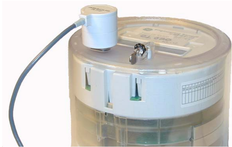
Figure 3.1 Optical port connection for kV2c meter
