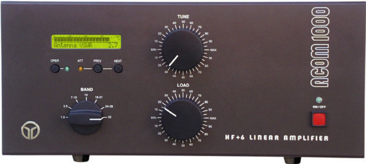
Fig.3-1 ACOM1000 Display and Control
