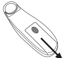
Slide the battery cover off the reverse of the remote control.
