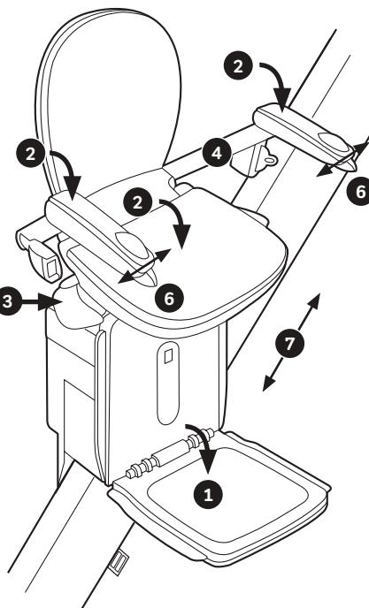
The Acorn 180 Curved Stairlift is a modular system, designed for easy assembly and maintenance utilising the rack and pinion method of travel along the rail, which is still the most reliable system available. This method is used with customer safety paramount throughout design and manufacture. You may experience some small bumps or jolts during use of the stairlift; this is normal for this type of technology
