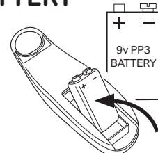
Insert the new battery base first and push down firmly to make.
