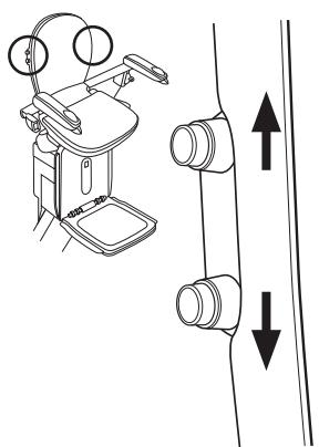
If a Powered Footrest is fitted, at the top or bottom of the stairs, after the stairlift comes to a stop, undo the seat belt and leave the stairlift.
