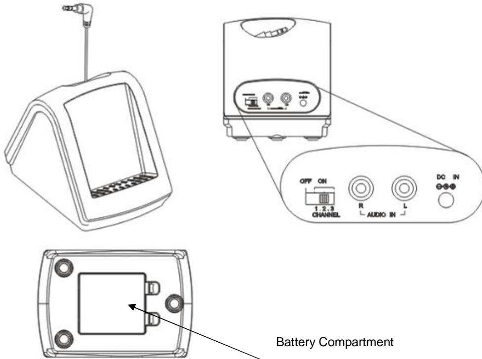
Turn the switch to On and the LED of transmitter will light up in Green. When the audio cable has been connected turn on the audio source to at least the mid range level and play the music. The LED will turn from Green to Blue (note: if the audio source is not in the play mode the LED will not turn from green to blue). If a speaker is not turned on within 4 minutes the transmitter light will turn from Blue back to green to save power.
