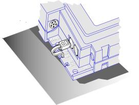
The internal modem (modulator/demodulator) converts electronic data into tones, which are then transmitted over phone lines.
