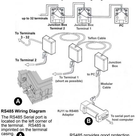
RS485 communication allows up to 32 terminals to be connected to one serial port. An RS232 port on the host PC is used with an RS232/RS485 converter to complete the connection.
