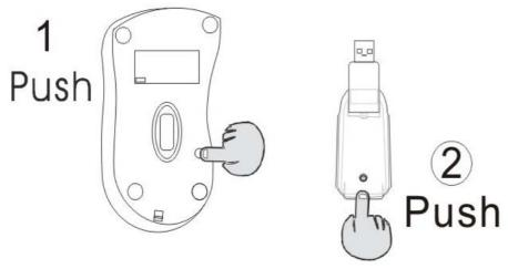
Push the channel reset button on the mouse. Push the channel reset button on the receiver If the cursor does NOT move after 30 seconds, please do the steps above.
