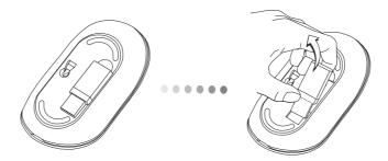
(B) Plug the USB receiver into an available USB port on your computer.
