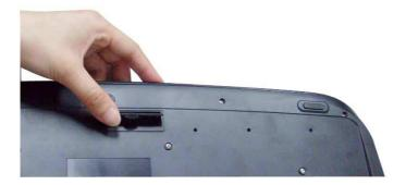
5. Install two AAA batteries into your keyboard following the battery orientation guide in the battery bay.
