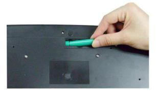
6. Replace the Battery Compartment Cover back onto your keyboard until it securely locks. The LED indicator on your keyboard will light up for 3 seconds after the batteries are installed successfully.
