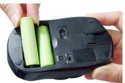
3. Replace the Battery Compartment Cover back onto your mouse until it securely locks.
