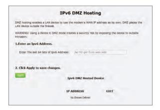
**Caution!** A DMZ host is not protected by the firewall and may be vulnerable to attack. Designating a DMZ host may also put other computers in the local network at risk. When designating a DMZ host, consider the security implications and protect it if necessary.
