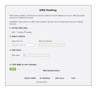
**Caution!** A DMZ host is not protected by the firewall and may be vulnerable to attack. Designating a DMZ host may also put other computers in the local network at risk. When designating a DMZ host, consider the security implications and protect it if necessary.
