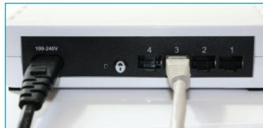
**Step 12** Plug the other end of the **Ethernet Cable** into the device that you want to connect to the Internet.
