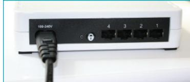
**Step 5** Plug the other end of the **Ethernet Cable** into an **OPEN Ethernet Port** on your Broadband Modem or Router.
